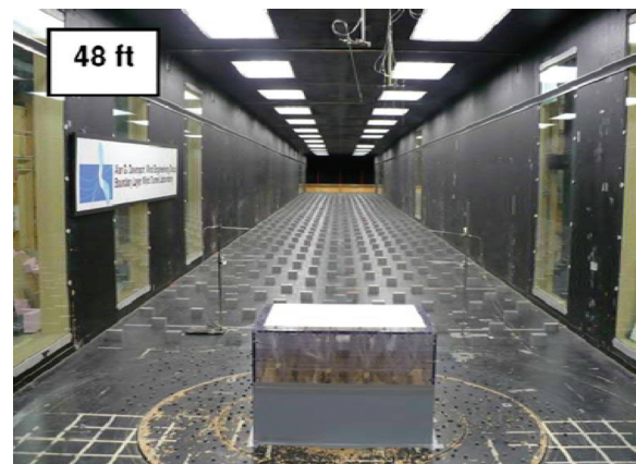
Figure 1: Boundary Layer Tunnel with building and rooftop solar array at UWO facility
